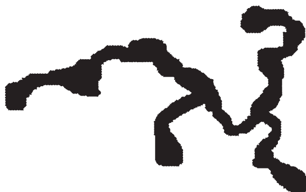
Figure 1 Structure of Ketjenblack EC-600 JD primary aggregate.
